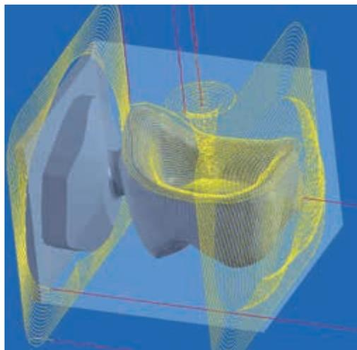
The machining of glass ceramic with traditional milling strategies places a great amount of strain on the milling tools, which are costly to replace. Specific grinding strategies are therefore required if the tool-life is to be optimized.
