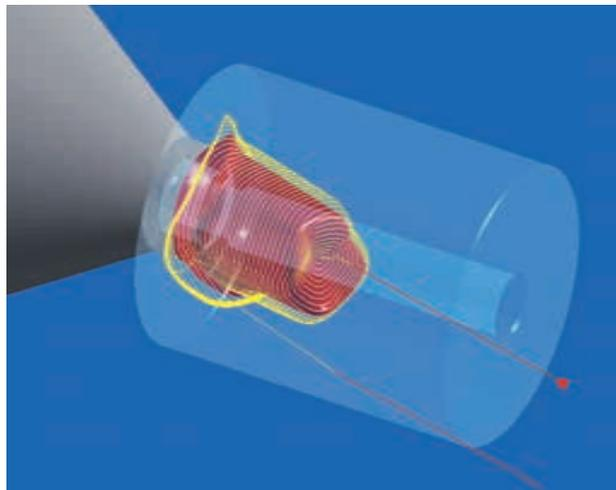
In the case of prefabricated abutments, the implant interface and screw channel have already been pre-milled, therefore, the lab or milling center only needs to finish the emergence, shoulder, and abutment body. This translates to faster manufacturing times, as the most intricate process has been completed. Additionally, *hyperDENT*® allows for prefabricated abutments to be milled using either multipart or single fixtures, providing even more flexibility and freedom of choice.
